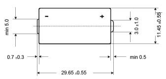
Dimensions are in millimeters and include label.
